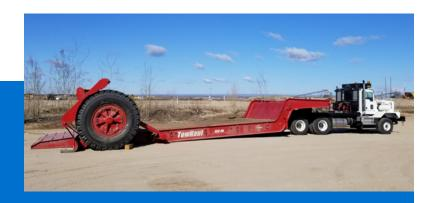
The TowHaul Rear-Loading Lowboy is purpose-built for rugged conditions, making it an excellent choice for dozers and small drills. Its compact and agile design ensures compatibility with various prime movers, such as articulated dump trucks, and heavy-duty over-the-road trucks.
